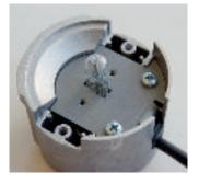
The contact surfaces between the lampholder and the luminaire housing combined with the thermally conductive metal plate on the lamp cap efficiently conduct the heat of the low-voltage halogen lamp, channelling it away to the housing.
