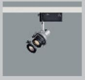
Pollux projector spotlights are available as a modular system or a complete product consisting of spotlight housing, anti-dazzle cone and holder with projection lens and mounting ring. Additional framing attachments can be mounted on the holder, gobos or structured lenses can be mounted on the mounting ring to project patterns. The individual elements can be adjusted and locked using the knurled screw on each carrier.
