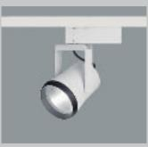
The floodlights with the Spherolit oval flood reflector are shaped so that they produce an axially symmetrical light distribution for floodlighting. The floodlights are available for low-voltage halogen lamps up to 100W/12V and metal halide lamps up to 70W.
