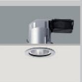
The directional luminaires are available in sizes 3 and 5. They are fitted with low-voltage halogen capsule lamps up to 100W/12V or low-volage halogen reflector lamps up to 35W/12V. The lampholder carrier can be tilted up to 15° and rotated through 360°.
