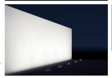
The optimum offset from the wall for the wallwasher is half of the wall height. The luminaire spacing can be set at up to 1.25 times the offset from the wall.
