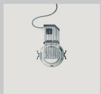
The housings of the recessed luminaries are cast aluminium and designed as heat sinks. The mounting rings, which are visible from below, are also cast aluminium, powder-coated white. Glare-free darklight reflectors are mostly aluminium and silver anodised. The product ranges available have cut-off angles of 30° and 40°. The luminaires can be fitted with two lamps of up to 2x42W.
