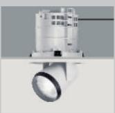
With the Spherolit technique for wallwashing, the reflectors are formed so as to produce an asymmetrical light distribution for wallwashing with focal emphasis in the upper area of the wall. The recessed Spherolit wallwashers are available for low-voltage halogen lamps up to 100W/12V, metal halide lamps up to 70W, and high-pressure sodium vapour lamps up to 100W.
