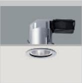
Directional luminaires are available in size 5. They are fitted with 35W or 70W metal halide lamps. The lampholder carrier can be tilted up to 15° and rotated through 360°.
