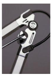
Functional luminaire design does not include superfluous elements and derives its quality from the technical necessities which is evident, especially in the design details. All Lucy task light hinges are made of solid cast aluminium and can be individually adjusted. Moulded plastic elements ensure that the exposed cables are held at the correct angles.
