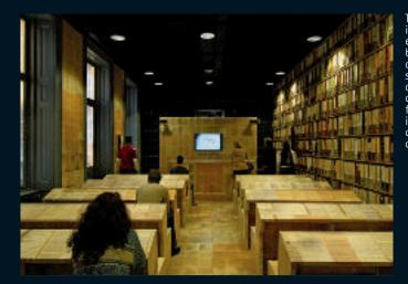
The use of surface-mounted downlights is often determined by practical considerations: For example, there might not be sufficient room to install recessed downlights in the ceiling. The conscious decision to use surface-mounted downlights in a lighting concept can considerably reduce installation costs, for example in buildings with solid ceilings or in existing buildings, the layout can be easily adapted to meet existing conditions.
