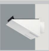
For Trion ceiling washlights for uniform ceiling illumination, double-ended QTDE12 tungsten halogen lamps up to 500W, or metal halide lamps up to 150W are to be used. Two cut-off shields provide variable control on the main axis of the luminaire, these can be freely adjusted.
