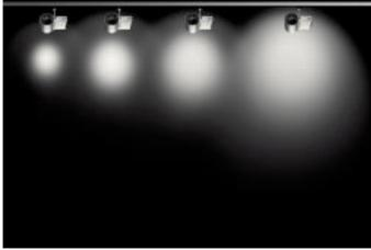
To ensure optimal illumination of both large and small objects. the spotlights are available with different beam angles. This allows designers to select the size that suits the distance to the object. The range of beam angles extends from narrow spot (< 10°) to spot (10°-20°), flood (25°-35°) and wide flood (> 45°).
