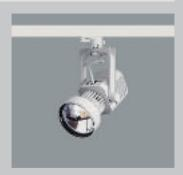
Eclipse spotlights are available for low-voltage halogen lamps up to 100W. They have electronic transformers and operation is confirmed by an LED function indicator. They can be dimmed using the integral potentiometers. High-pressure discharge lamps with 35W are also
