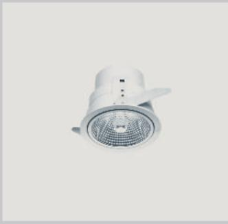
The housing and the mounting ring are of white plastic. The luminaire is closed off by a safety glass. The aluminium Darklight reflector is mirror-finish silver anodised. Assembly without tools is facilitated by the fixing springs at the side. The necessary control gear is available as an accessory. The luminaires have a cut-off angle of 30°. An anti-dazzle cap attached to the non-reflecting safety glass prevents glare from the lamp providing visual comfort.
