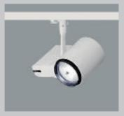
With Spherolit technology for wall-washing, the reflectors are formed so as to produce an asymmetrical light distribution for wallwashing with focal emphasis in the upper area of the wall. The Spherolit wallwashers are available for low-voltage halogen lamps up to 100W/12V and metal halide lamps up to 150W.
