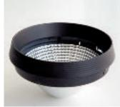
Anti-dazzle ring The black plastic anti-dazzle ring provides optimum visual comfort. Together with the reflector, it forms a single unit that attaches to the spotlight housing with a bayonet fixing.
