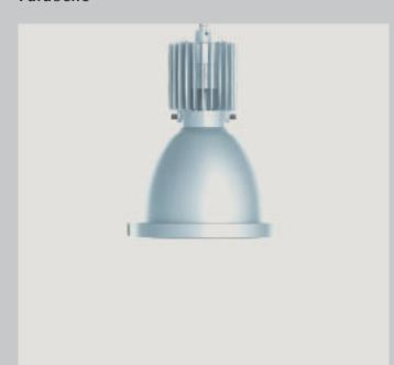
The housings are cast aluminium or aluminium extrusions and powder-coated silver. The surfaces are designed as heat sinks. The visible, glare-free Darklight reflectors are also made of aluminium and silver anodised. The cut-off angle is 40°. The lower reflector edge is finished off by a cover ring painted silver on the outside and black on the inside. The pendant downlights are available in sizes 8 and 10. Pendant tubes, wire ropes, spiral cables and safety glasses are available as accessories.
