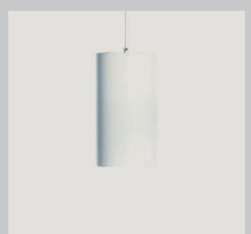
The cylindrical housing is aluminium and powder-coated white. Glare-free Darklight reflectors are aluminium and are silver anodised. The cut-off angle is 40°. When suspended a white pendant tube is used and the electrical connection to the ceiling is concealed within the small white plastic canopy.
