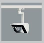
Jilly floodlights are available in four housing sizes. An anti-dazzle frame in black powder-coated cast aluminium limits the emission of light. Tungsten halogen lamps up to 500W, operated via 3-circuit adapters, are to be used. The control gear for metal halide lamps up to 70W and the electronic control gear for compact fluorescent lamps up to 42W are contained within the transadapters.
