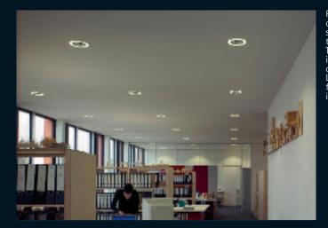
Recessed luminaires are completely subordinate to the light they emit. They are so fully integrated in the ceiling that they hardly register as a design feature. The most important factor determining the effect created by space and objects is the play of light on surfaces. Light emitted by downlights can vary from very narrow beams to diffuse wall illumination.
