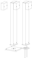
The Kubus can be mounted to suit any situa tion using ERCO's range of acces-sories: a mounting plate, a post, a base, and a concrete anchor.
