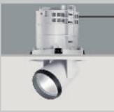
The oval flood Spherolit reflector is designed to produce an axially symmetrical light distribution for floodlighting. The recessed floodlights are available for low-voltage halogen lamps up to 100W/12V, metal halide lamps up to 70W, and high-pressure sodium vapour lamps up to 100W.
