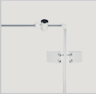
The product range consists of profile section lengths of 2m to 4m. The 36mm x 72mm rectangular sectioned aluminium profile is available silver or powder-coated white. The underside is designed as a 3-circuit track and the topside as an empty compartment or as a luminaire. The light structure's connectors are suitable for forming linear and rightangled layouts. Pendant tubes or wire ropes are available as suspension systems.
