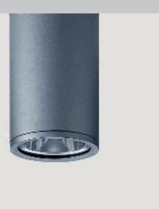
Cylinder surface-mounted downlights are suitable for both outdoor and indoor use. The housings and the screw-mounted cover rings with safety glass are made of cast aluminium, provided with a special coating and double powder-coated in the shade Graphit m. Glare-free darklight reflectors are aluminium and silver anodised. The cut-off angle is 30°. The high-quality reflectors are protected against the ingress of dust and dirt of any kind.
