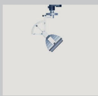
The product range consists of spotlights, floodlights and lens wallwashers. The transformer housing, bracket and luminaire head are cast aluminium, powder-coated white or silver. The electrical connection is made using a 3-circuit adapter or a DALI adapter. Pinions running on gear wheels with printed graduations enable the angles of rotation and tilt to be selected and locked.
