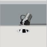
The Quintessence directional luminaires are available in the Spherolit reflector versions spot or flood. The luminaires above the darklight reflector with a cut-off angle of up to 40° can be tilted up to 30° and rotated through 360°. The range comprises luminaires in sizes 3 to 7 for metal halide lamps up to 150W or 100W high-pressure sodium vapour lamps.
