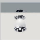
The downlights are used for low-voltage halogen lamps up to 50W/12V or metal halide lamps of 20W. In the downlight version only the frosted glass cover is visible. The transformers or control gears required are to be ordered separately. Concrete housings, plaster rings and cover rings are available as accessories.
