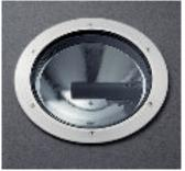
Tesis adjustable uplights combine high visual comfort and a particularly shallow installation depth. To enable precisely placed grazing light on facades – despite any inaccuracy when installing in the ground, the uplights' narrow light beam can be adjusted by a few degrees tilt.
