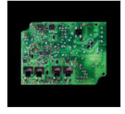
Modern control gear Electronic control gear provides greater comfort than conventional control gear and is more efficient. It is smaller, protects the lamps and is a far more environmentally friendly option. ERCO only uses lead-free soldered
