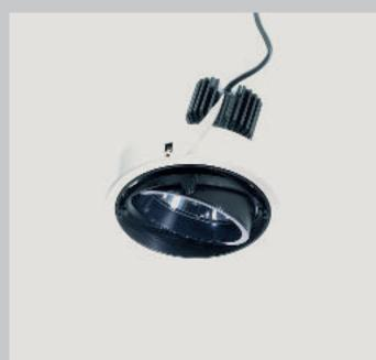
Gimbal recessed spotlights are cardanically suspended and the joints are made of black powdercoated cast aluminium and black plastic. The white mounting rings are plastic. The luminaires' cardanic suspensions in the mounting ring allows a tilt of up to 40° in almost all directions.
