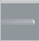
ERCO 3-circuit track is available in lengths up to 4m. When connected to a three-phase network, each of the three circuits can be loaded to a maximum of 16A. The circuits must be separately protected. In the DALI version, one conductor carries the phase and the two others are used for the information signal. All the connectors for 3-circuit installation or for DALI applications are available for making the electrical connection.
