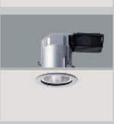
The directional luminaires are available in size 5. They are fitted with high-power LEDs in warm white or daylight white. The lampholder carrier can be tilted up to 20° and rotated through 360°.
