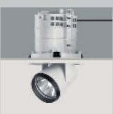
Logotec recessed spotlights have attachments that can be removed without tools for quick lamp replacement. The various Spherolit reflectors produce very narrow to wide light distribution. The spotlight range in two sizes features low-voltage halogen lamps up to 100W/12V, metal halide lamps up to 70W and high-pressure sodium vapour lamps up to 100W.
