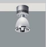
The downlights are used for low-voltage halogen lamps up to 50W/12V. The surface-mounted downlight features a visible, cyl-indrical transformer housing with built-in electronic transformer.
