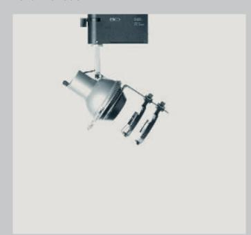
Pollux spotlights consist of a housing with cast aluminium bracket. They are available in white and silver. The electrical connection is made using a transadapter with LED function indicator and potentiometer to adjust the brightness. Low-voltage halogen lamps up to 50W/12V are to be used. The brightness can be adjusted from 10%-100% on the transadapter using the integral potentiometer. The 20W metal halide lamp is used in all Pollux spotlights and lens wallwashers.
