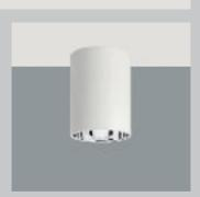
Surface-mounted downlights are available in sizes 5, 7 and 8 for various lamps. Halogen reflector lamps QPAR20 50W or QPAR30 up to 100W, metal halide lamps 70W or compact fluorescent lamps TC-DEL 26W are to be used.
