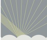
Spherolit reflectors ERCO's patented reflector technology optimally combines visual comfort and efficiency. Due to the different shapes of the computer-calculated spherolites on the reflector surface, the reflector characteristics can be
