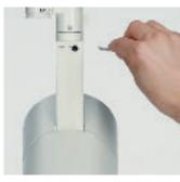
The small "lock" screw on the Parscan spotlights simultaneously locks the luminaire rotation and the tilt with just one turn. This locks the position of the luminaire in situations where luminaire arrangements are frequently changed. For wallwashers, it ensures that the beam direction remains unaltered when a lamp is replaced; to ensure the quality of the lighting concept is maintained.
