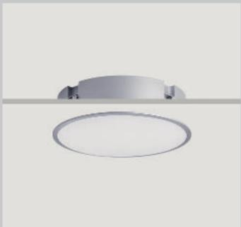
The housings of the Panarc product range are all plastic and are available in white or silver. Flood lenses or prism lenses and diffusers direct the light and act as the lamp retainers. The necessary control gear for the operation of lamps is contained within the housing. Concrete housings, plaster rings and cover rings are available as accessories. All Panarc luminaires meet IP44 protection mode.
