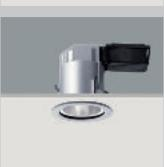
A directional luminaire is available in size 5. A QPAR30 100W is used here. The lampholder carrier can be tilted up to 15° and rotated through 360°.
