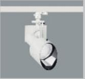
Lens wallwashers are available for low-voltage halogen lamps up to 100W/12V and high-pressure discharge lamps up to 150W. Each lens wallwasher is fitted with a wallwasher attachment. This includes a spread lens and the typical ERCO wallwasher reflector.
