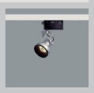
Low-voltage halogen reflector lamps up to 50W/12V are to be used. An anti-dazzle ring functions as a lamp retainer. The LED function indicator and the potentiometer to adjust the brightness are on the transadapter for low-voltage halogen lamps. A version for the metal halide lamp of 20W with Spherolit reflector is also available. The tilt and rotate motions are provided through the
