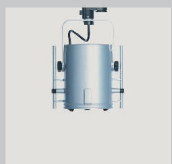
The range consists of three spotlight sizes. The housings are cast aluminium and powder-coated black, white or silver. The lateral guides are used to mount accessories. The electrical connection is made using a 3-circuit adapter or transadapter with integral electronic transformer. For low-voltage halogen lamps and high-pressure discharge lamps, a safety glass covers the lamp.
