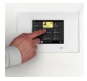
The Light Changer is a control panel featuring touch screen technology providing access to the stored light scenes. The clear and convenient user guidance provides for easy daily operation.
