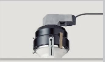
The housings are cast aluminium and designed as heat sinks. The mounting rings, which are visible from below, are also cast aluminium, powder-coated white. Glare-free darklight reflectors are aluminium and silver anodised. The cut-off angle is 40°. Tubular metal halide lamps 35W, 70W and 150W are used as lamps. The necessary control gear for the operation of the lamps is available as an installa-tion unit that is operated independ-ently in the ceiling void. It must be ordered separately.
