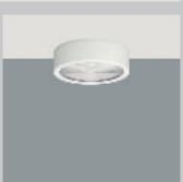
The downlights are available in two housing sizes. Depending on the version, compact fluorescent lamps 2x9W, 2x18W or 1x36W are to be used. The lamps are arranged horizontally, resulting in a very shallow installation height. A rotationally symmetrical beam is produced with the flood lens.
