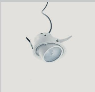
Compar recessed spotlights can be rotated up to 360° and tilted by 30°. The housings are cast aluminium. The mounting rings, which are visible from below, are also cast aluminium, powder-coated white. The Spherolit reflectors with a facetted surface are also aluminium and silver anodised. The inside of the anti-dazzle ring is powder-coated black. The necessary control gear for the lamps have to be ordered separately. The directional luminaires can be mounted without tools.
