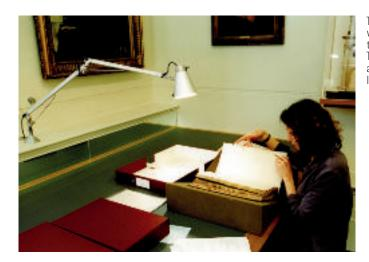
The luminaires are provided with hinges to allow flexibility to suit any lighting requirement. The Fresnel lens or spread lens as lamp cover ensures optimum light distribution.
