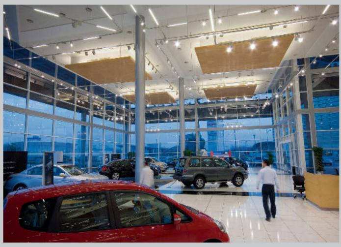
With a 50mm tube diameter, Monopoll light structures provide a good solution wherever a filigree lighting system is required which remains subordinate to the architecture. T16 fluorescent lamps are to be used in direct luminaires as well as in the wallwasher.
