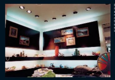
Recessed spotlights combine the flexibility of spotlights with the discreet appearance of recessed luminaires. Their main application is accent lighting. Tilt mechanisms allow the luminaires to be aimed both at objects and vertical surfaces. Recessed spotlights are inconspicuous architectural details and can ideally be combined with downlights.
