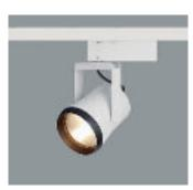
72424.000 White (RAL9002) DALI **72474.000** Silver DALI QT12-ax 100W 12V GY6.35 2200lm Spherolit reflector, oval flood
