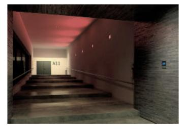
The Multichrome version of the uplight allows space to be recreated with different colours of light. The flood light distribution means that coloured, scenic lighting effects can be projected uniformly across a ceiling. Due to the spectral properties of coloured fluorescent lamps, all the colours of light produced have a pastel character.
