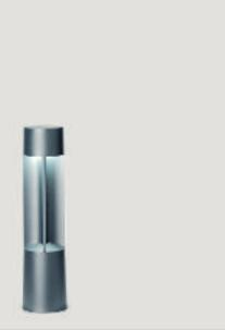
Panorama bollard luminaires rated to protection mode IP65 are ideal for outdoor lighting applications. The housings are provided with a special treatment which is followed by a double powder-coating in Graphit m. The lens system of the luminaires is covered with a safety glass to protect them against the ingress of dust and dirt. The control gear is integral within the luminaire housings and these luminaires can be mounted on a ground socket, a concrete anchor or a mounting plate.
