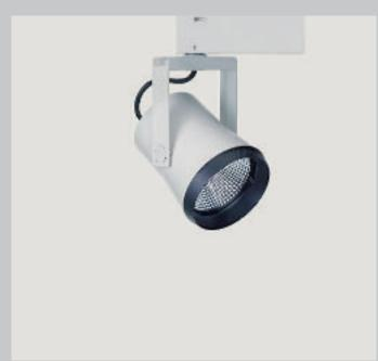
The Logotec range includes spotlights, floodlights and Spherolit wallwashers in two sizes. The housings are made of cast aluminium and powder-coated in white and silver. The electrical connection is made using a Transadapter. DAL1-compatible luminaires feature a DAL1 transadapter. Amongst the accessories are colour filters and filters to reduce both IR and UV radiation.
