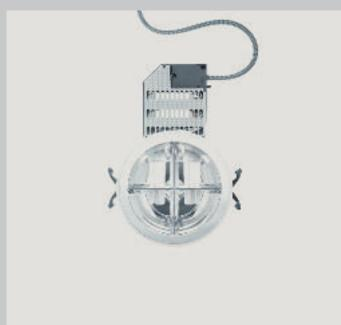
The housings of this range are cast aluminium and designed as heat sinks. The mounting rings, which are visible from below, are also cast aluminium and powder-coated white. The lampholders are positioned to lie horizontally. The necessary control gear is usually mounted on the side of the housing. If several luminaires are installed then separate control gear is available.
