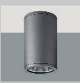
Surface-mounted directional luminaires are available in size 5 with LEDs, for low-voltage halogen lamps, PAR lamps or metal halide lamps. The lampholder carriers can be tilted up to 20°. Some directional luminaires are fitted with a sculpture lens which changes the round beam into an oval.
