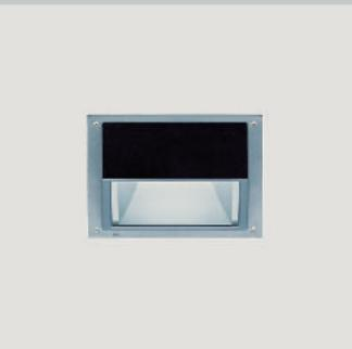
Paratec luminaires are offered in three sizes, accordingly named Paratec I to Paratec III. These are designed for recessed mounting in walls or ceilings. The housings are high-quality cast aluminium provided with a special coating. Over this, a double powder-coating is applied. The triangular portion of the housing is visible below the ceiling. The double powdercoating is available in graphit m and white. Clear safety glasses act as luminaire cover.
