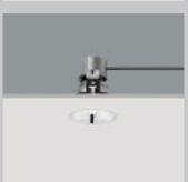
The double washlights are available in sizes 4 and 5 for low-voltage halogen lamps up to 100W. The Spherolit reflector has two special wallwasher segments for uniformly illuminating parallel walls whilst simultaneously lighting the room.
