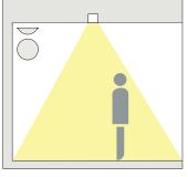
light is emitted to the sides, the possibility of dazzling the observer is minimised.
