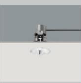
The washlights are available in sizes 4 and 5 for low-voltage halogen lamps up to 100W. The darklight reflector has a special wallwasher segment in Spherolit technology for illuminating walls whilst simultaneously lighting the room.
