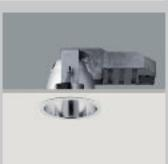
This product range includes downlights with electronic control gear and darklight reflectors in sizes 5 to 10. The necessary control gear is mounted on the side of the housing. Concrete housings, plaster rings, cover rings and mounting rings for flush ceiling mounting or mounting plates for plank ceilings are available as accessories.
