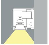
The small version of the Cylinder facade luminaire is intended exclusively to emit light vertically downwards.
