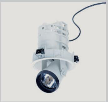
The Logotec range includes recessed spotlights, recessed floodlights and recessed Spherolit wall-washers in two sizes. The luminaires can be operated in four installation positions and tilted by 90° as well as rotated through 360°. The housings are made of cast aluminium and powder-coated in white. Amongst the accessories are colour filters and filters to reduce both IR and UV radiation.
