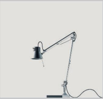
The product range consists of three light heads of silver-lacquered aluminium. They have cast aluminium lampholder carriers designed as heat sinks containing the control switch. The light heads can rotate and tilt on the rigid arm. Two aluminium arms are connected together by a hinge and a visible connecting strut, this together with internal springs provides stabilisation. The integral cables are only visible at the hinged joints.
