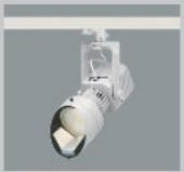
Using low-voltage halogen lamps up to 100W/12V or 35W highpressure discharge lamps allows a uniform illumination of walls in rooms up to 6m high. Each lens wallwasher is fitted with a wall-washer attachment. This includes a diffusing lens and the typical ERCO wallwasher reflector.
