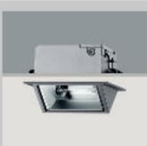
Depending on size, version and connected load, double-ended tungsten halogen lamps up to 300W or metal halide lamps up to 150W. The necessary ECGs are integrated inside the housings. The reflector system allows wallwashing up to 12m high with uniform illuminance distribution.
