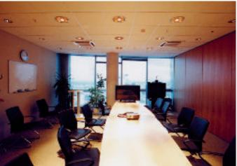
The combination of fluorescent lamps and low-voltage halogen lamps in one luminaire housing provides a choice between economical and uniform illumination or an atmosphere defined by accent lighting. The fluorescent lamp component produces a wide light distribution.
