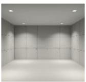
30° cut-off angle Quintessence luminaires with a cut-off angle of 30° achieve high vertical illuminance with highly uniform illuminance on the floor even with low ceiling heights. This cutoff angle provides sufficient glare
