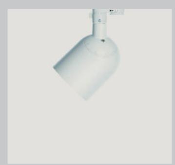
The product range is available in three cylinder sizes of varying diameter and length. The housings are powder-coated white. The adjusted angle of tilt can be read off from the graduated scale. The electrical connection is through the ERCO track adapter.
