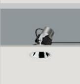
The Quintessence directional luminaires are available with spot or flood Spherolit reflector. The luminaires above the darklight reflector with a cut-off angle of up to 40° can be tilted up to 30° and rotated through 360°. The range comprises luminaires in sizes 3 to 5 for low-voltage halogen lamps up to 100W.
